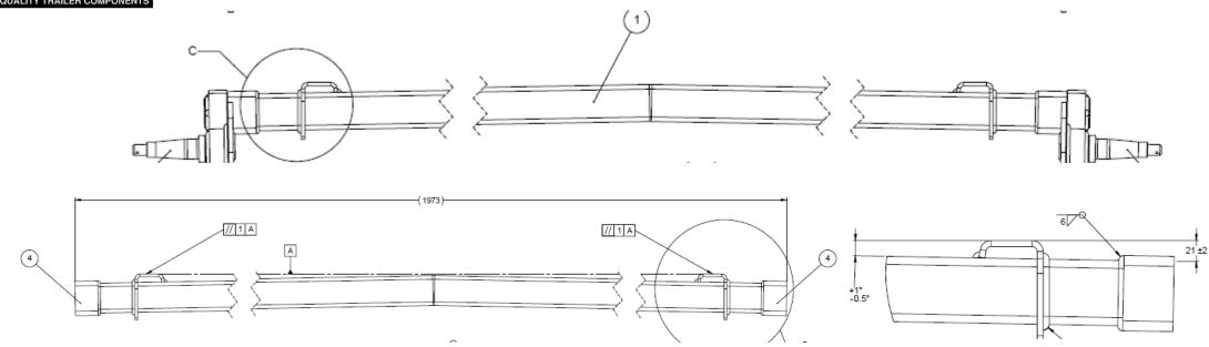
Trojan Duratorque trailer axles are designed with a "bend" in the tube that will deflect when the load (weight of the trailer) is applied. This will bring the trailer wheel camber toward a 0 value that is the best setting for most trailer applications. This will allow the tyres to wear evenly and allow the longest tread life.
